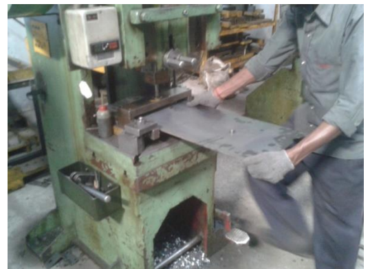
Piercing with locating pins and stoppers
