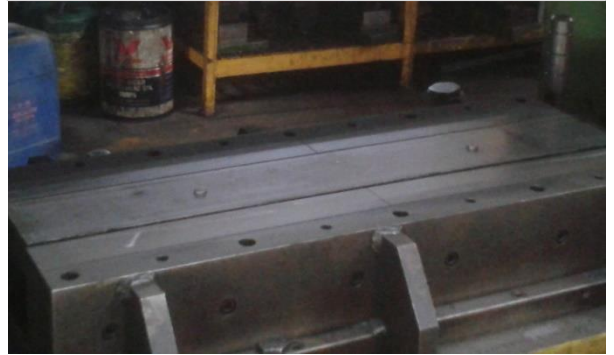
Die for Drawing/Bending with locating pins
