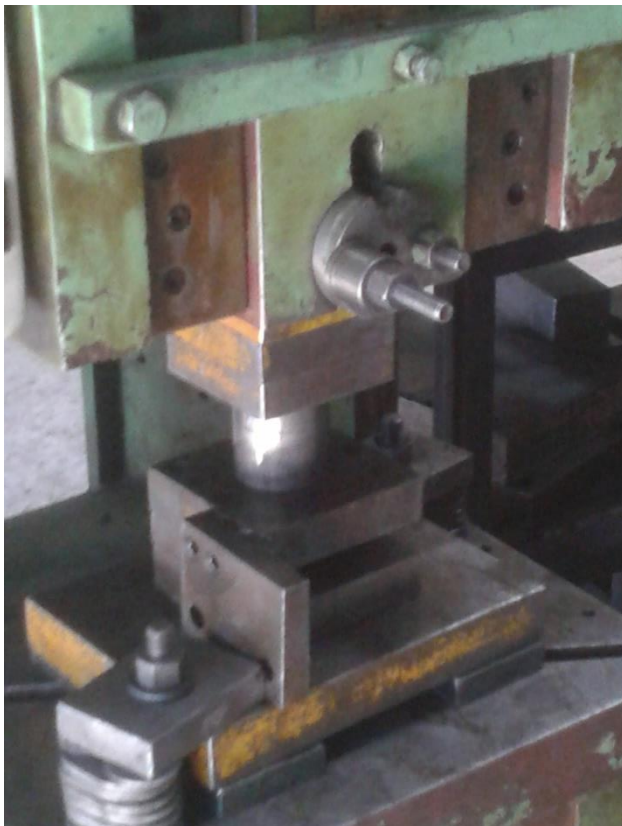
Notching tool with stopper
